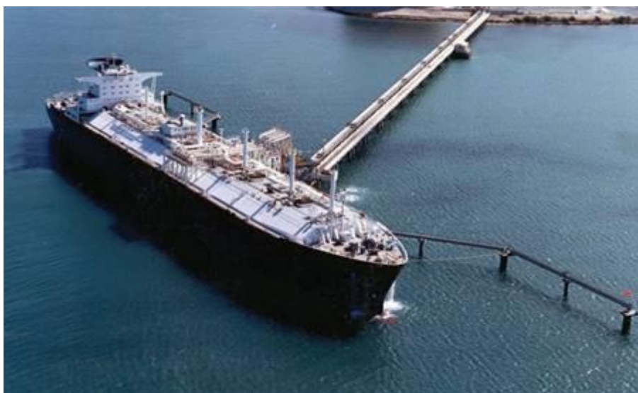
Figure 2-14 LNG Carrier with Membrane Tank System
