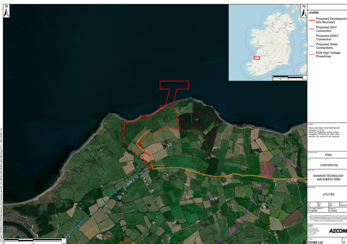
Figure 2-22 Proposed Electrical and Water Connections
