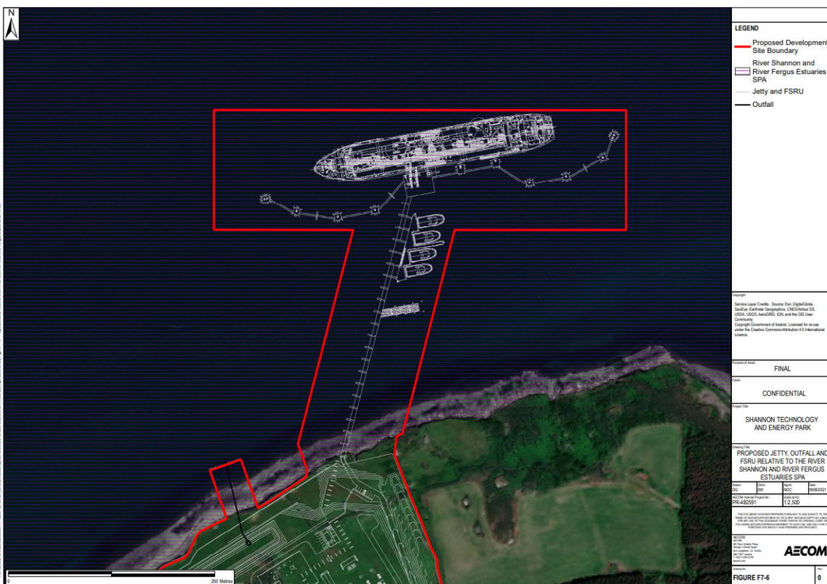
Figure 7A-4 Proposed Jetty, Outfall and FRSU Relative to the River Shannon and River Fergus SPA
